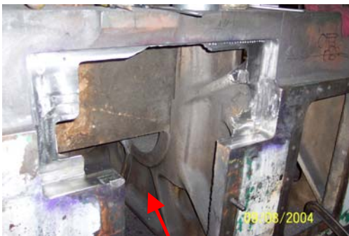
Broken out window on a large compressor frame
