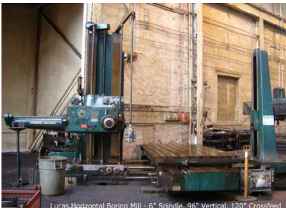
Lucas Horizontal Boring Mill - 6" Spindle, 96" Vertical, 120" Crossfeed
