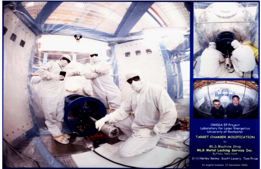
On-site machining of 2 EP & 1 Omega Flange
