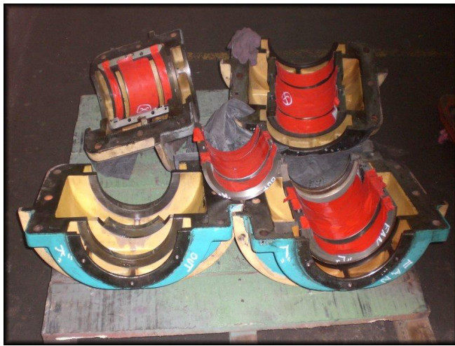
Bearing Cap Machining - Added Vibration Sensors
