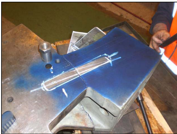
Preparing the area for a masterlock to affix foot on locomotive engine
