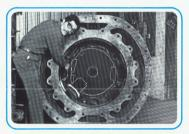
Pieces were cast and machined to fit and replace the entire broken area. Sections then were metal laced and sealed against pressure, sufficient to restore the piece to full working load. Using broken ram (above) for pattern, a new and stronger ram was cast locally and machined in our shop.
