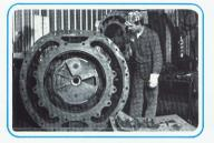
Above are the results of freeze breaks in a 4200 C.F.M. air compressor with a 755 horsepower motor. High-and low-pressure cylinders and heads were shattered in water jacket areas. Photo shows low-pressure head (note broken pieces in foreground) prior to repair.
