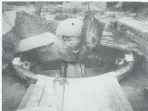
SPIDER OF GYRATORY STONE CRUSHER REPAIRED ON LOCATION
