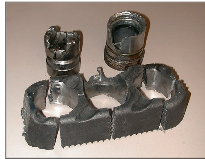
Damaged cam, aluminum liner, and crosshead guide (note center section)
