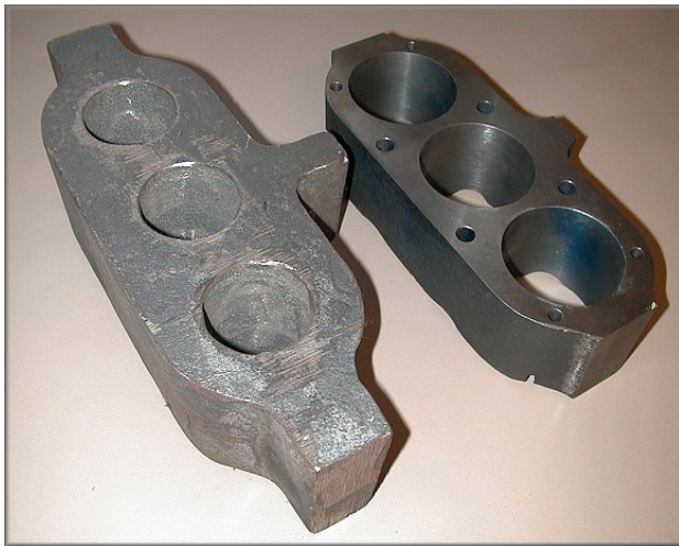
Rough casting (left side) and finish machined casting (right side)
