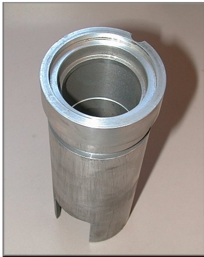
Typical Aluminum Liner used for alignment
