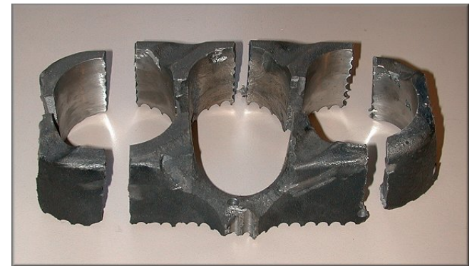
Damaged casting removed via drilling along a plane and removing with an air chisel
