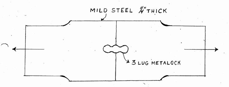
Comment - This test showed that a 3 lug lock will not give satisfactory holding strength for a metalock repair of any type.
