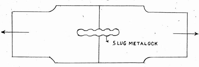
Comment - The failure occurred because the lugs of the metalock and the restrictions of the steel plate deformed under compression and shear. The lock therefore pulled out intact. Poor workmanship in forming the locking channel in the steel plate caused this failure below the ultimate strength of the lock.
