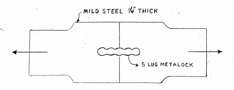
Comment - The failure occurred because the lugs of the metalock and the restrictions of the steel plate deformed under compression and shear. This point failed at the average strength of the Metalock
