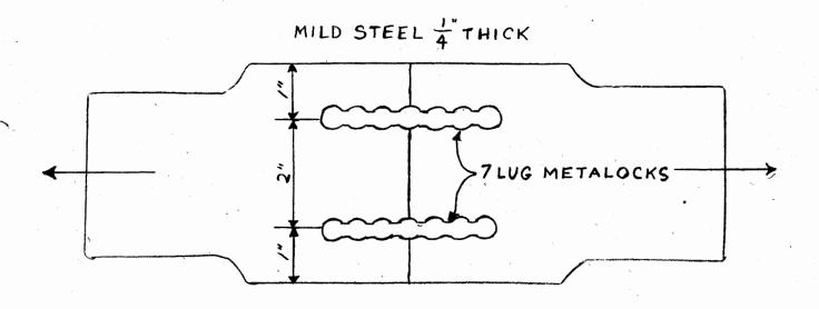
Comment - The failure occurred because the locks pulled out of the restrictions in the steel plate, the locks remaining intact. The side thrust caused by the pressure of the lugs against the restrictions in the steel plate developed the moment sufficient to bend out the side sections of the plate thereby releasing the metalock. This allowed a reduction in the ultimate strength of the joint.
