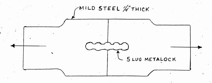
Comment - The restrictions and lugs of the metalock held firmly in place within the mild steel plate and no preceptible movement occurred between the lock and the plate. The ultimate tensile strength of the lock was below average (5400 lbs.)
