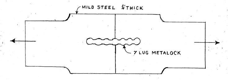
Comment - The restrictions and lugs of the metalock held firmly in place within the mild steel plate and no perceptible movement occurred between the lock and the plate. The ultimate tensile strength was beyond the average (5400 lbs.). for a 1/4 x 1/4 metalock due to good workmanship and a very strong lock.
