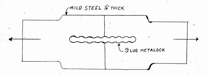
Comment - The restrictions and lugs of the metalock held firmly in place within the mild steel plate and no preceptible movement occurred between the lock and the plate.
