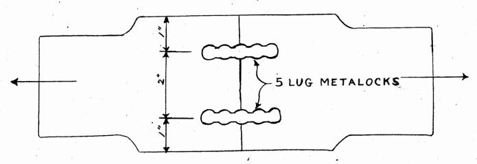
Comment - The failure occurred because the locks pulled out of the restrictions in the steel plate, the locks remaining intact. The side thrust caused by the pressure of the lugs against the restrictions in the steel plate developed a moment sufficient to bend out the side sections of the plate thereby releasing the metalock. This allowed a reduction in the ultimate strength of the joint.
