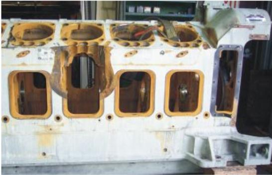
Crankcase Window damage occurs when a connecting rod fails and becomes wedged between the window and the crankshaft. The window is typically blown outward resulting in local crosshead guide damage. This is our most demanding repair as alignment of the replacement piece is critical for correct operation.
